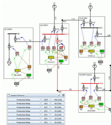
**Detecting deceptive real-time automation controller with out-of-band reporting**
