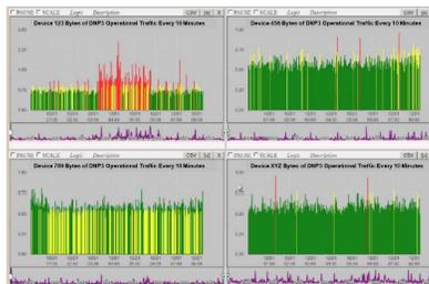
**Example TrafficProfiler time series SCADA indicators**
