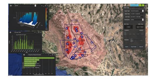
SUMS calculates, validates and maps accurate, verified spectrum usage and occupancy metrics to address spectrum-related operational questions such as where and when additional use of spectrum can be allowed or must be excluded.
